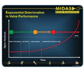
Given that we know this, it is possible to use Acoustic Emissions (AE) technology, for example, for guick and easy leak detection.
